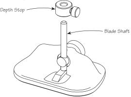
Figure 1: Installing the depth stop.
