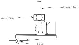
Figure 2: Setting depth stop.
